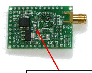
Remove R7 to enable the UART TTL signaling on pins 8-11. This will disconnect pins 13-16 from the UART interface.
