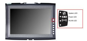
This device is equipped with different status LEDs in the front. These LEDs indicate current events, like the system activity state, the current accumulator charge status and WLAN activities.
