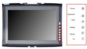
The keys on the front panel are occupied with the following functions by a specific driver in the soft keyboard:
