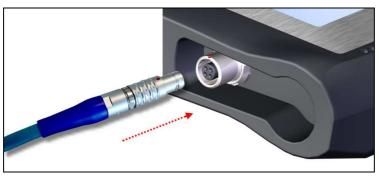
For disconnecting the SD Connect cable, it must be pulled rearwards in the area marked in green. This loosens the snap-in mechanism at the end of the plug.
