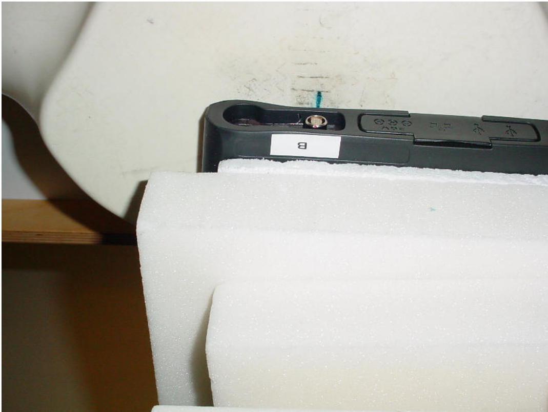
Photo 12: Test position front edge without any distance (antenna B)
