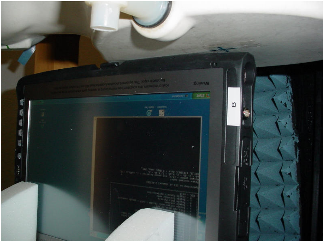
Photo 12: Test position front edge without any distance (antenna B)
