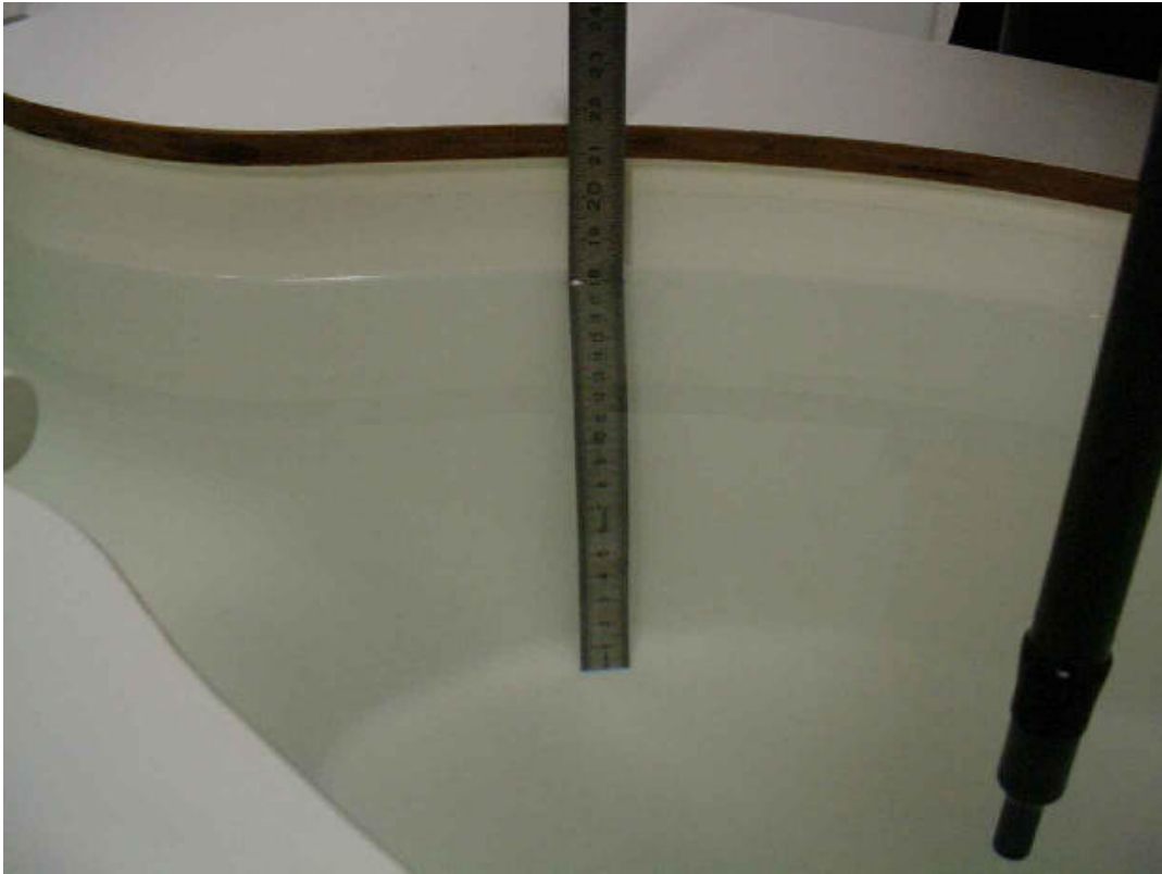
Photo 14: Liquid depth 5 GHz body simulating liquid
