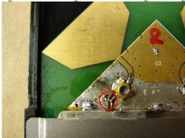
(3) Tied digital ground and analog ground together for removal of low frequency spurs.
