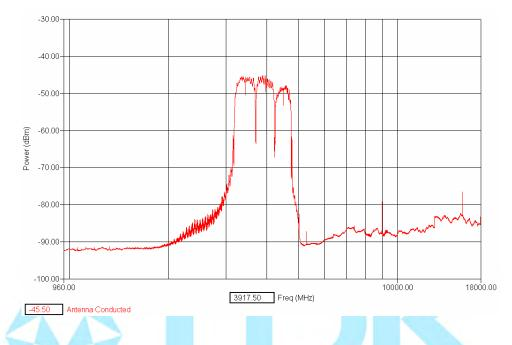
Conducted antenna port measurement made with 1 MHZ RBW / 3 MHz VBW
