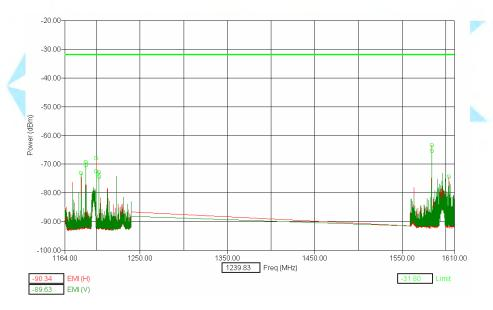
Measurements made with 10 kHz RBW / 10 kHz VBW at 1 meter distance.
