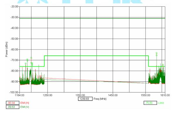
Lower limit line is 47 CFR, Part 15 sub part F
