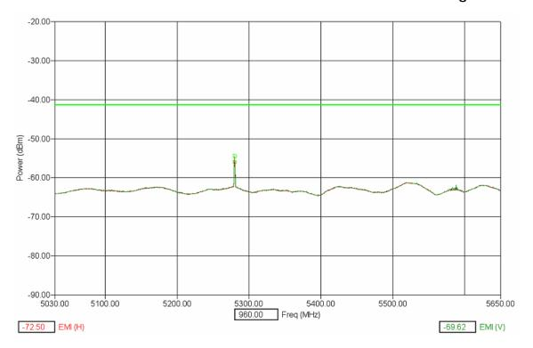
Measurements made with 1 MHz RBW / 3 MHz VBW at 1 meter distance
