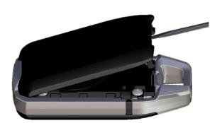
2. Insert 4"Coin" into the dent in 3"Coin battery cover", turn 90 degrees counterclockwise so that the OPEN position comes to  $\nabla$ , and remove 3"Coin battery cover".
