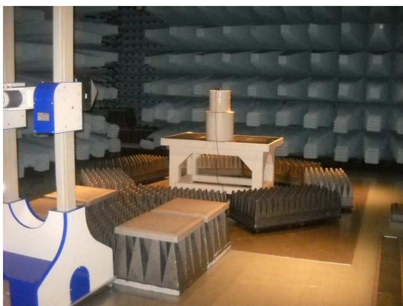
Figure 9.2-2: Radiated emission testing above 1 GHz
