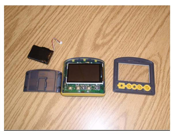
Photo Description: Front panel & display removed
