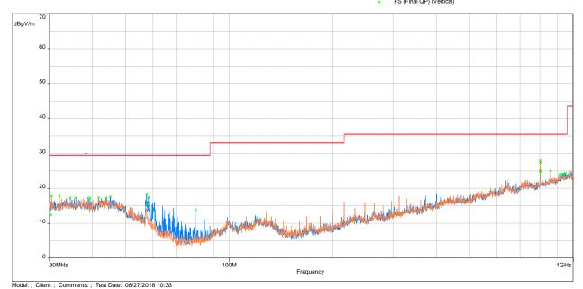
Lim. QPeak **Frequency** QPeak@10m Margin **Angle** Height Antenna Correction (MHz) (dBµV/m)  $(dB\mu V/m)$ (dB) **Polarization** (dB) (°) (m) 30.398 12.35 29.50 -17.15 3.13 Horizontal -9.53 46 801.811 27.29 35.50 -8.21 327 3.44 Horizontal -3.49 57.995 15.34 29.50 -14.16 58 3.96 Vertical -15.65 60.599 13.26 29.50 -16.24 177 3.35 Vertical -16.51 80.023 13.75 29.50 -15.75 292 3.60 Vertical -20.24
