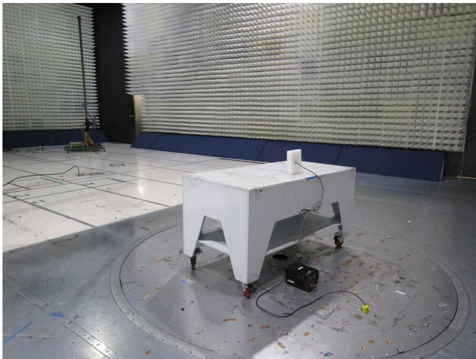
Electromagnetic Radiated Disturbance Setup Photograph
