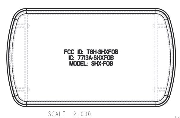
FCC ID AND IC NUMBERS, AND MODEL TO BE MOLDED INTO THE PART IN THIS GENERAL LOCATION. FCC ID: T8H-SHXFOB, IC: 7713A-SHXFOB, AND MODEL: SHX-FOB MUST BE LEGIBLE ON FINISHED PART ON THE SIDE SHOWN
