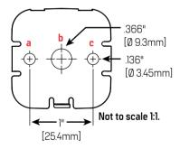
**NOTE:** Mounting plate **(B)** may be used as a drilling template.
