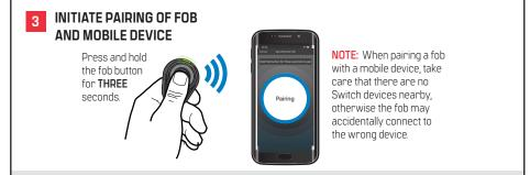
Press and hold the fob button for **THREE** seconds. The fob and mobile device should begin pairing. The fob LED will appear solid **green** for **ONE** second while searching for a device.
