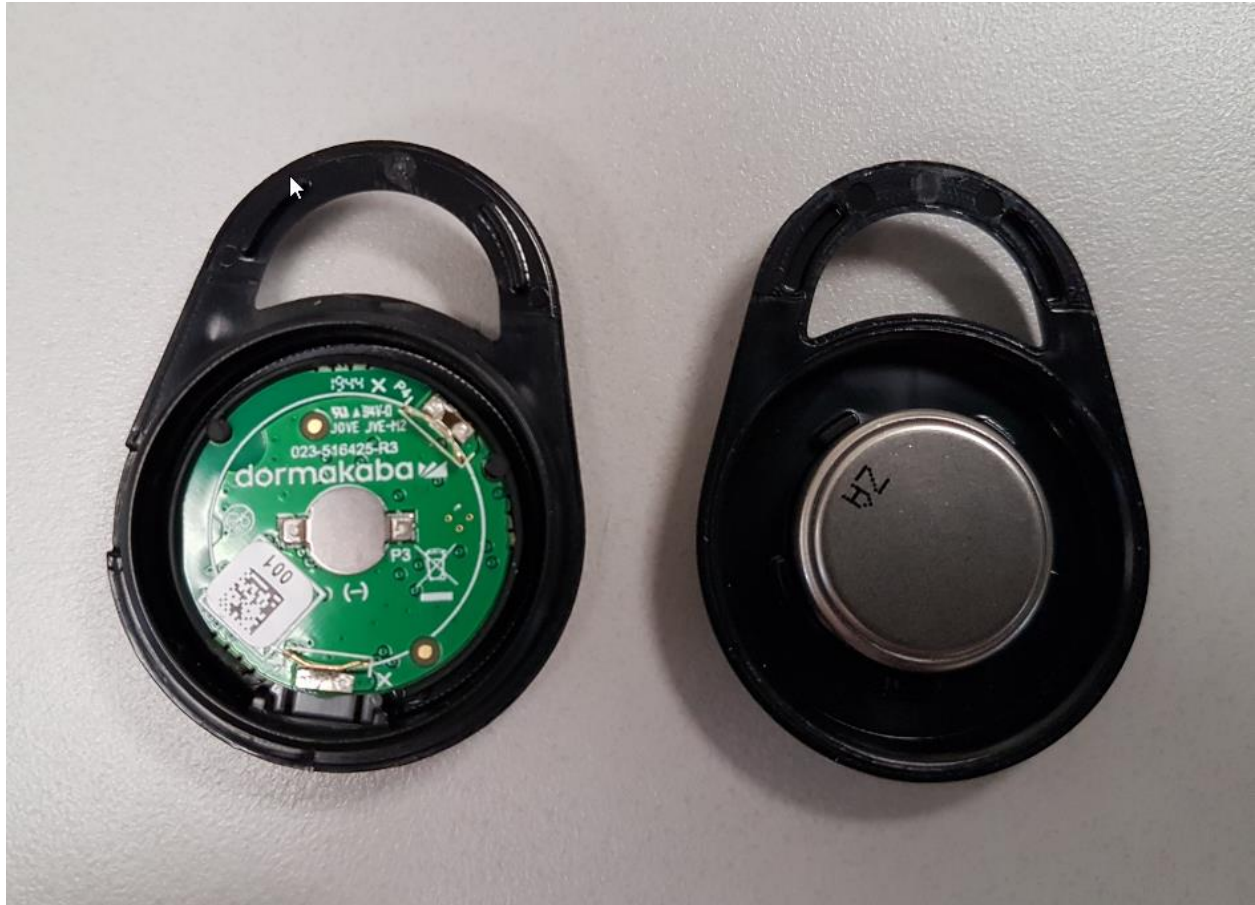
Figure 1- Open Fob with PCB and coin cell battery inside
