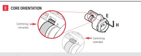
The hex key (H) should come inserted in the core (E) with the control lug retracted. If so, go to step 5. Otherwise, go to step 4 to retract the control lug.
