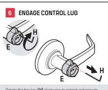
Rotate the hex key **(H)** clockwise to extend and engage the control lug. Remove the hex key **(H)**. Gently pull on the knob to ensure that the core **(E)** is properly installed.
