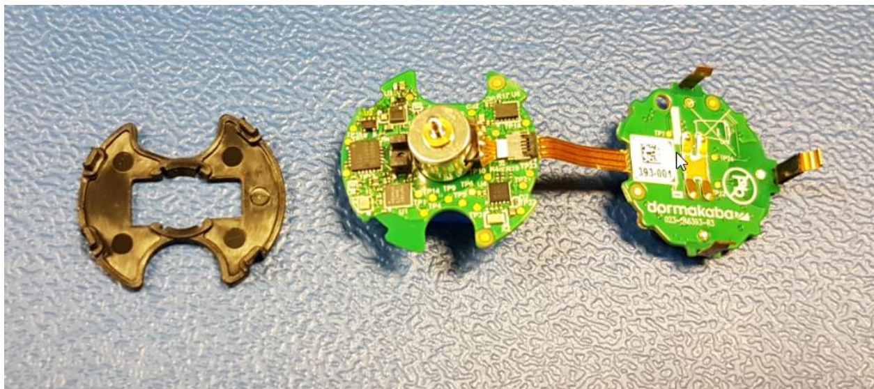
Figure 7- Switch Core PCB with Motor
