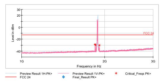
The peaks above the limit are the Carriers frequencies of the 3G Band II and LTE Band 25.
