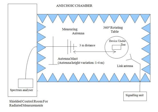
Radiated measurements above 1 GHz up to 8.5 GHz:
