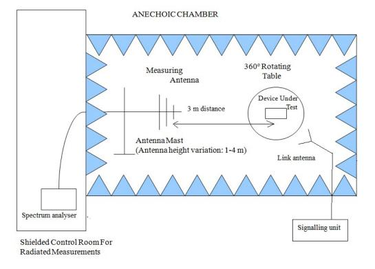
Radiated measurements setup from 1 GHz to 18 GHz:
