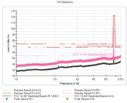
The peak above the limit is the carrier frequency.
