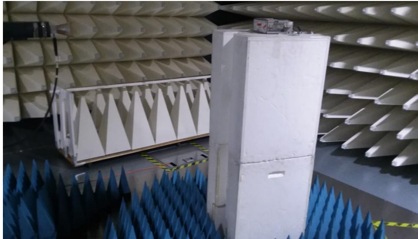
Figure C5. Radiated Emission High Range 18-40GHz test setup
