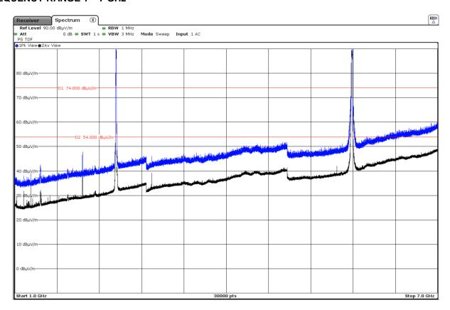
The peaks above the highest limit are the Bluetooth EDR, WLAN 2.4 GHz and WLAN 5 GHz carrier frequencies.
