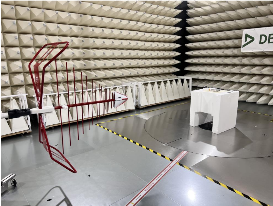
Figure C5. Low Range Radiated Emission test setup
