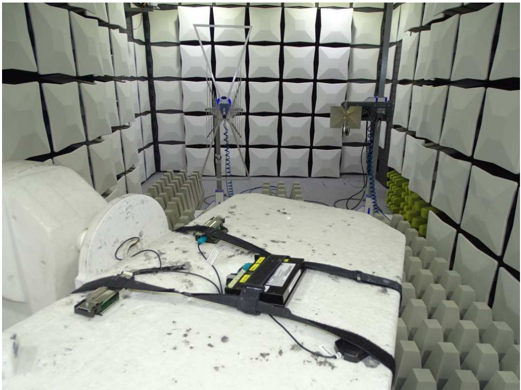
Photo 4: Test setup for radiated measurements (above 1 GHz)
