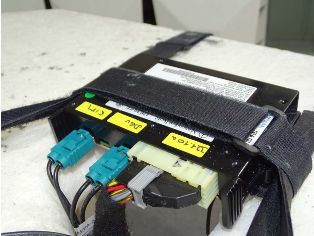
Photo 3: Test setup for radiated measurements (above 1 GHz)
