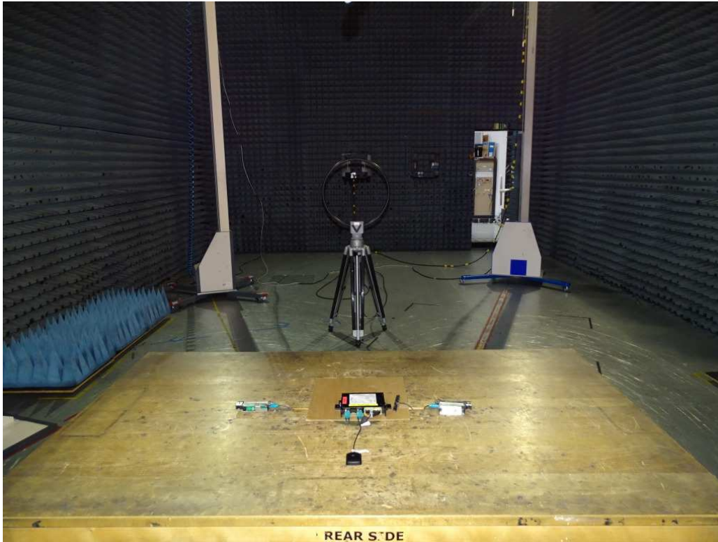
Photo 1: Test setup for radiated measurements (below 30 MHz)
