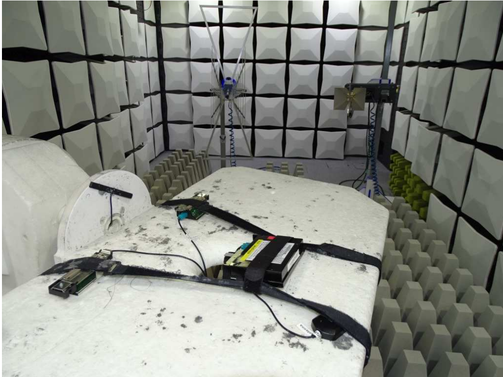
Photo 3: Test setup for radiated measurements (above 1 GHz)
