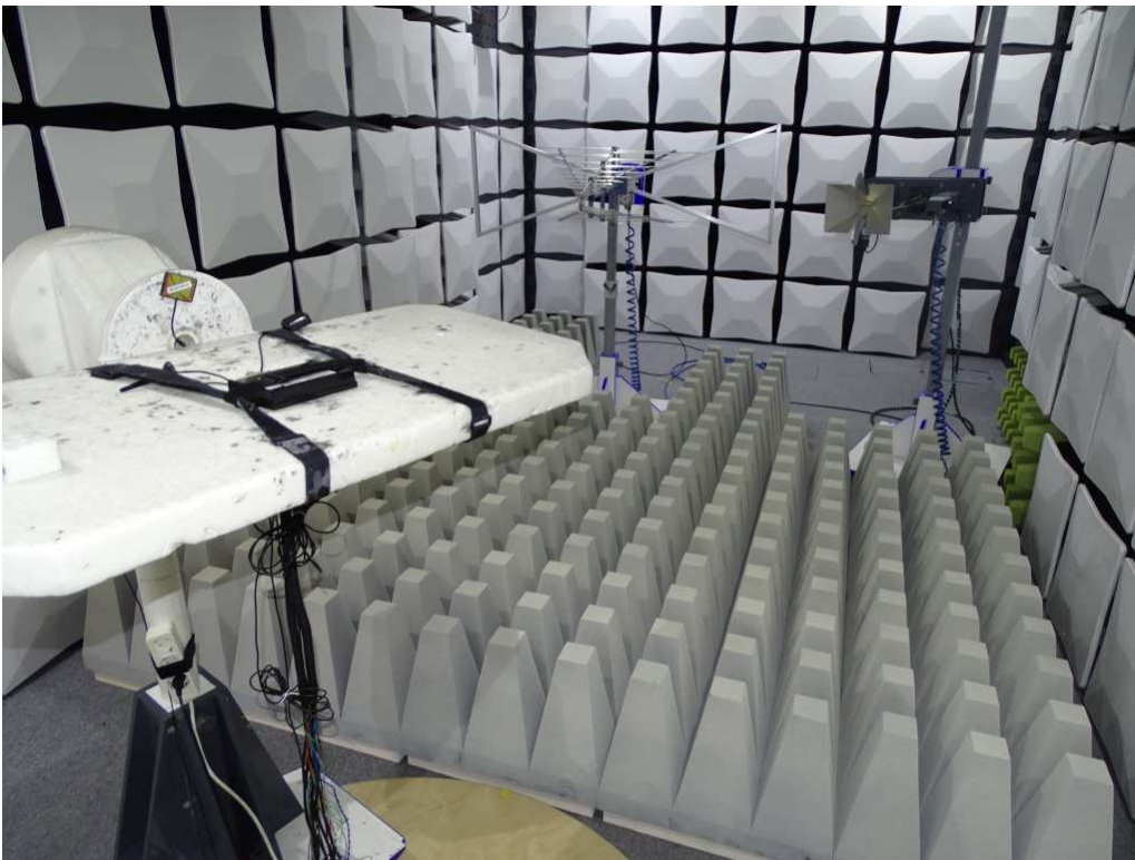
Photo 3: Test setup for radiated measurements (above 1 GHz)
