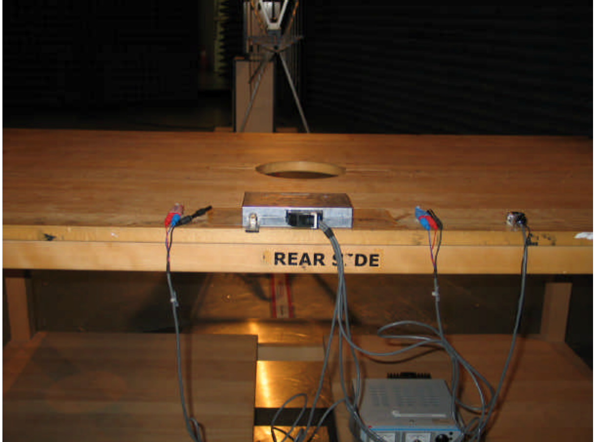
Photo 1: Test setup for radiated measurements below 1 GHz
