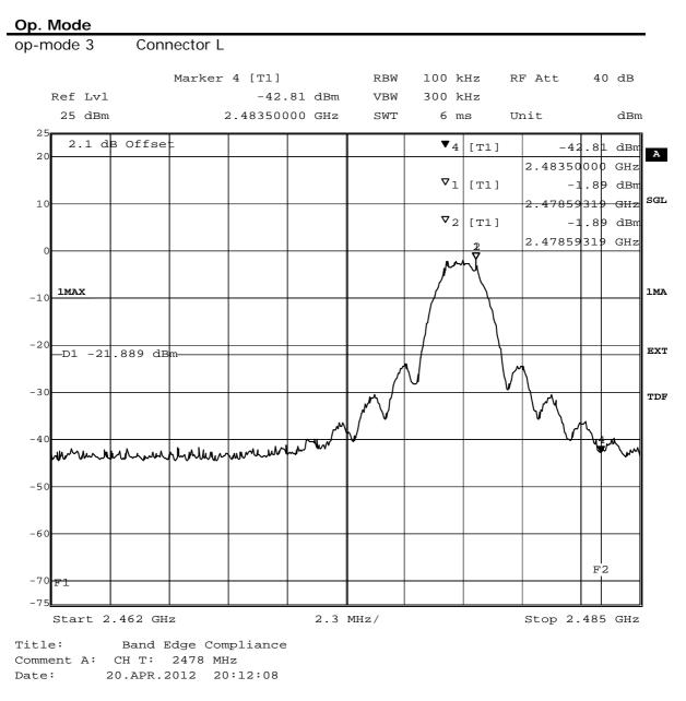
(band edge compliance, conducted measurement, higher band edge)
