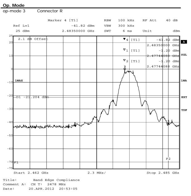
(band edge compliance, conducted measurement, higher band edge)
