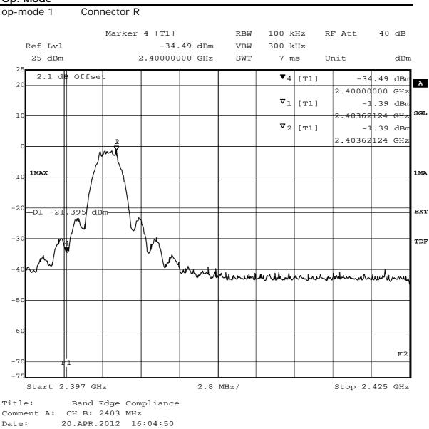
(band edge compliance, conducted measurement, lower band edge)
