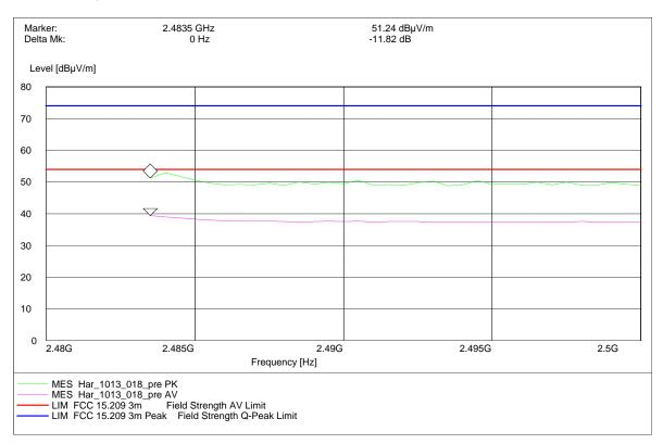
Radiated measurement (higher band edge)
