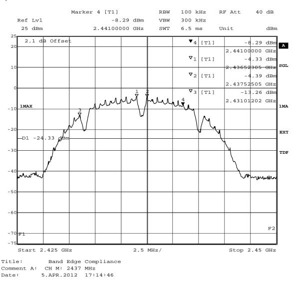
(determination of reference value for spurious emissions measurement)
