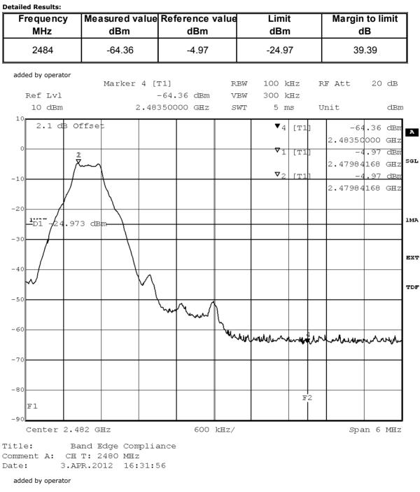
Test: 15c.6; Frequency = 2480, Mode = BT transmit using 1 Mbps with GFSK modulation, Method = radiated
