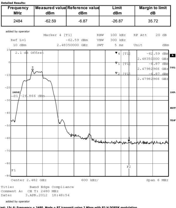
Test: 15c.6; Frequency = 2480, Mode = BT transmit using 2 Mbps with PI/4 DQPSK modulation, Method = radiated
