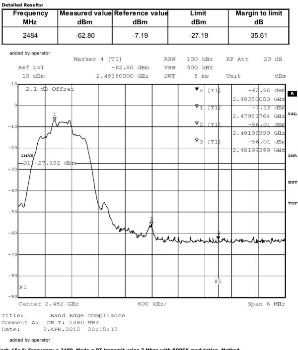
Test: 15c.6; Frequency = 2480, Mode = BT transmit using 3 Mbps with 8DPSK modulation, Method = radiated
