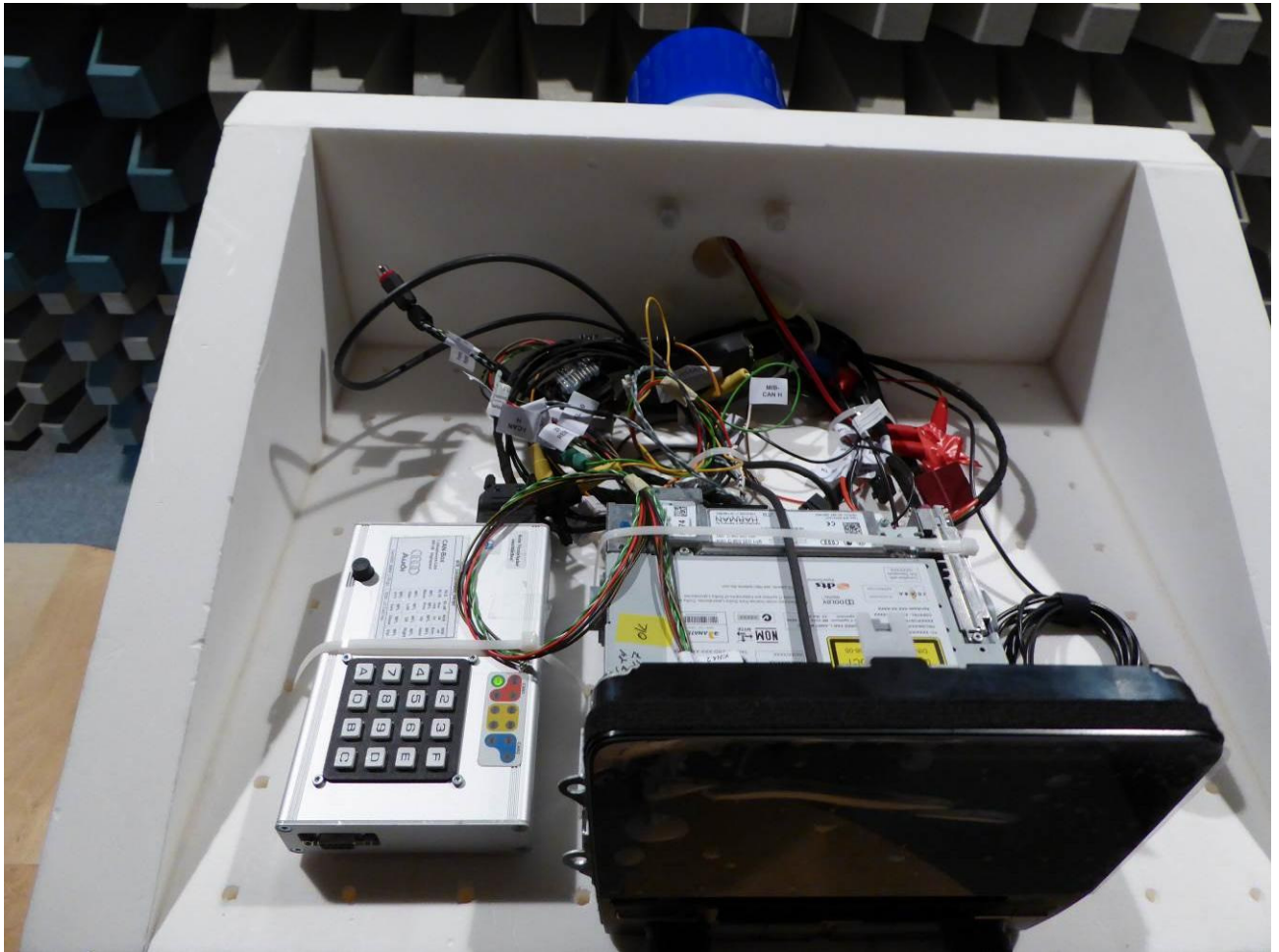
160090_39.jpg: Test setup - Radiated emission > 1 GHz (fully anechoic chamber)
