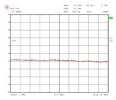
No significant frequencies above the noise floor of the system were found during the preliminary radiated emission test, so no measurements were carried out on the outdoor test site.
