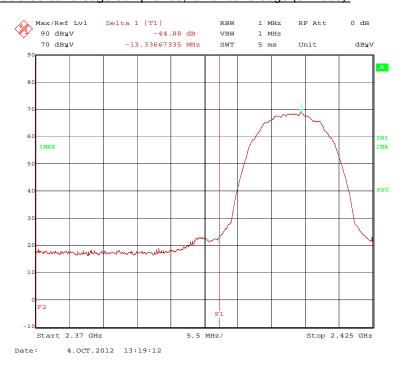
123736 14.wmf: Radiated band-edge compliance, lower band edge (q-mode):
