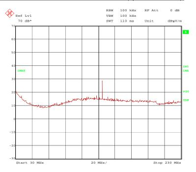
The following frequency was found inside restricted bands during the preliminary radiated emission test: 134.556 MHz.
