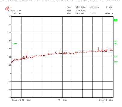
The following frequencies were found outside the restricted bands during the preliminary radiated emission test: 349.871 MHz, 888.096 MHz and 948.697 MHz.
