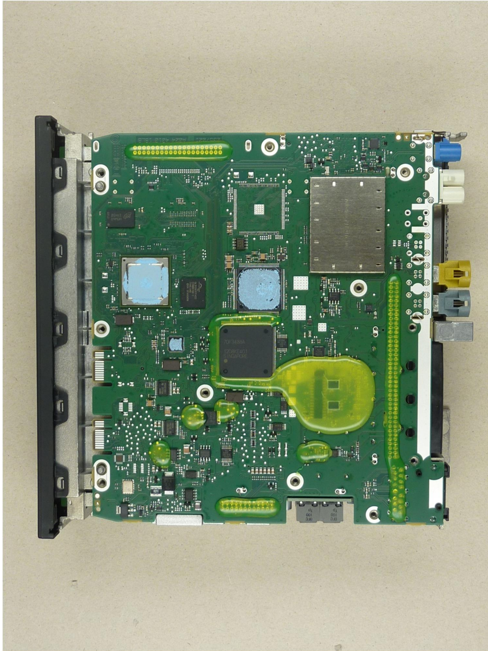
123736_31.JPG: Audi MIB, main PCB, bottom view
