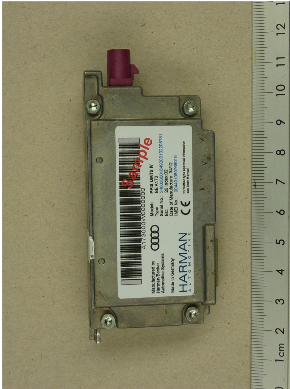
123736_27.JPG: UMTS module, top view
