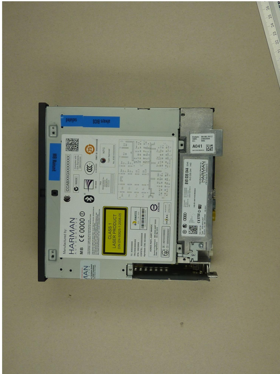
123736_28.JPG: Audi MIB, top view with removed UMTS module
