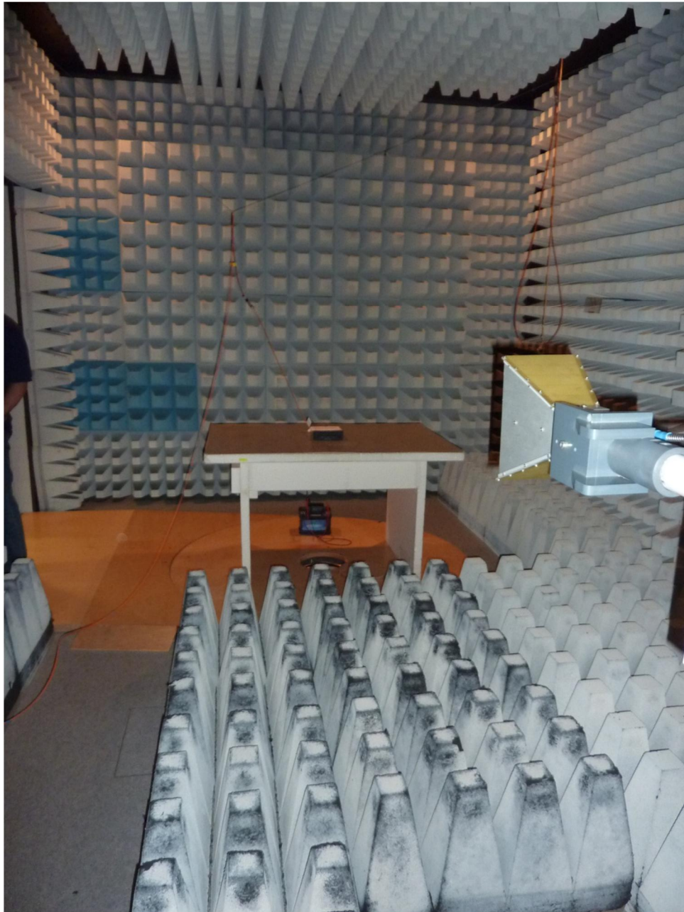
123736_3.JPG: Test setup fully anechoic chamber
