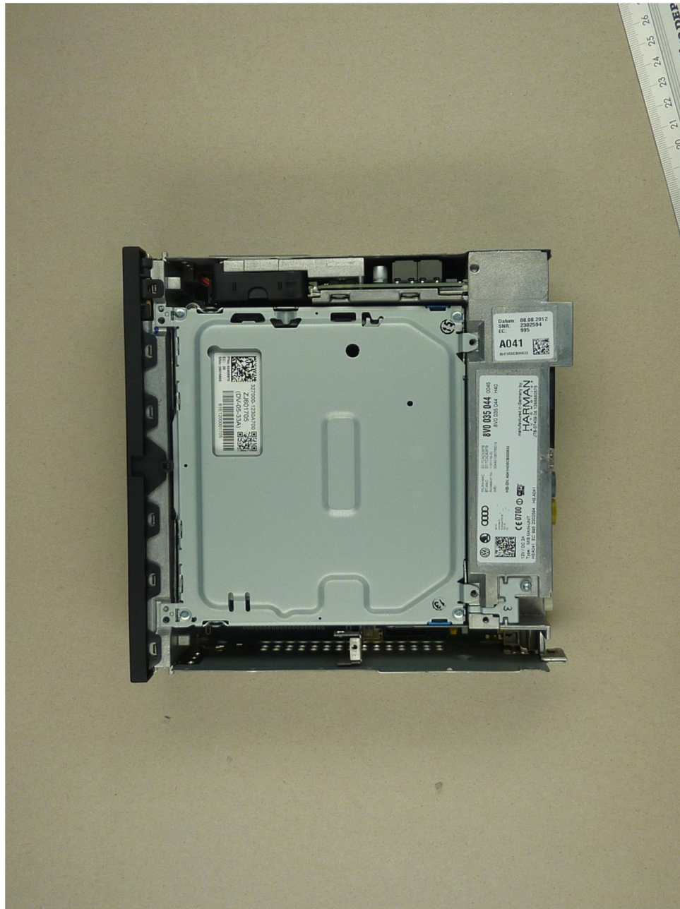
123736_29.JPG: Audi MIB, top cover removed
