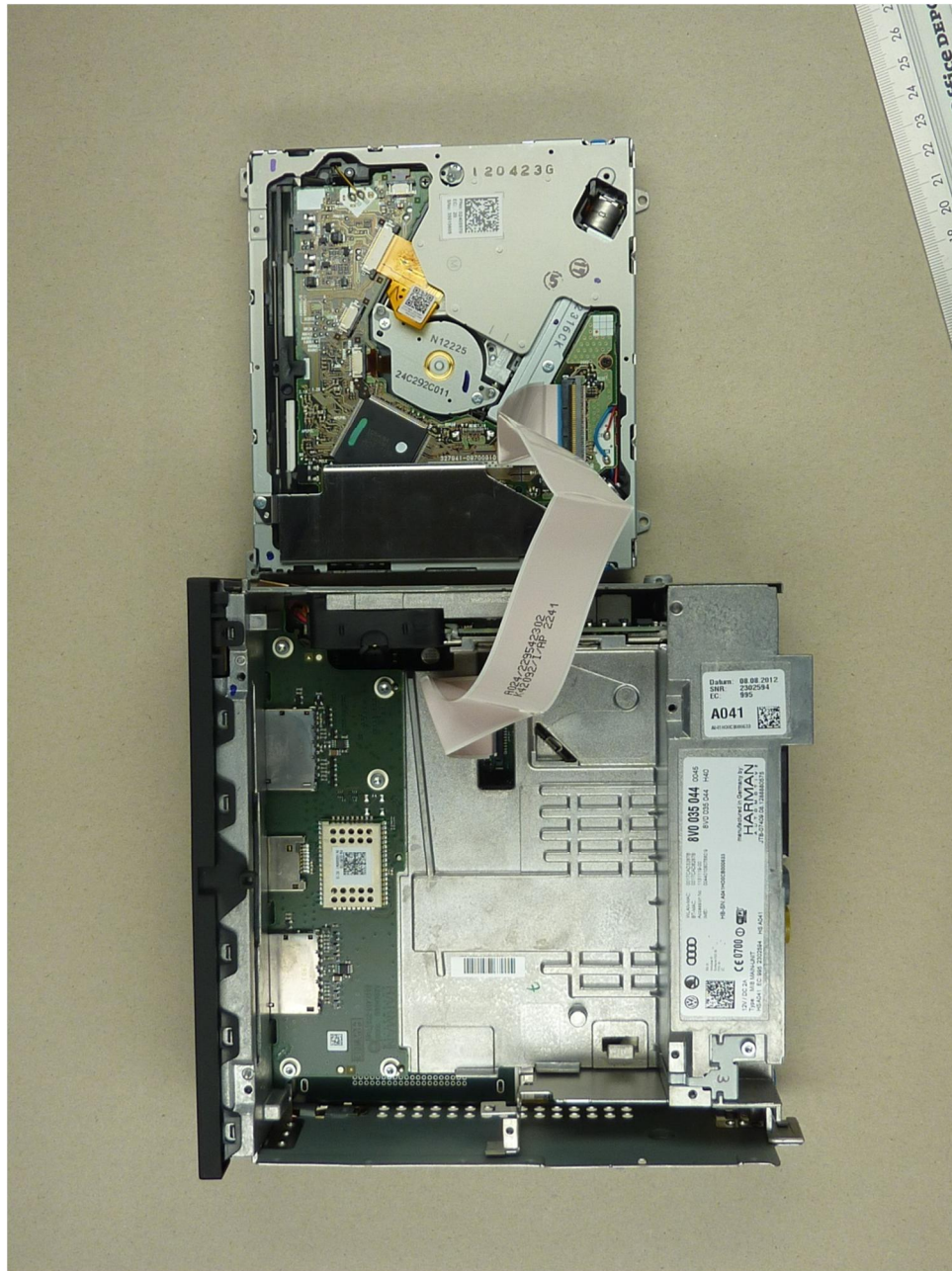
123736_30.JPG: Audi MIB, CD/DVD drive removed, top view
