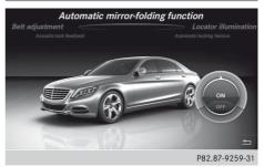
If the function "Automatic folding mirror function" is switched on, the exterior mirrors fold in automatically as soon as you lock the vehicle from the outside and then fold out again when you unlock it.
