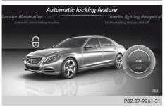
When the automatic locking feature is activated, the vehicle is locked automatically when the ignition is switched on and the vehicle is travelling faster than walking pace.
