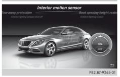
When the interior motion sensor is primed, a visual and audible alarm is triggered if movement is detected in the vehicle interior. This can occur if someone reaches into the vehicle interior, for example.
