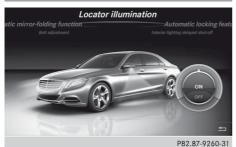
If the locator illumination (surround lighting) is switched on, as well as the turn signals, the headlamps will also light up briefly when the vehicle is unlocked.
