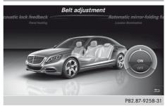
The seat-belt adjustment function adjusts the driver's and front-passenger seat belt to the upper body of the occupants.
