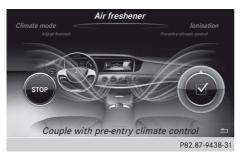
You can connect the perfume atomiser with the pre-entry climate control, i.e. the atomiser switches on together with the pre-entry climate control.
