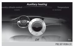
You can pre-set three departure times for automatic activation of the auxiliary heating. To select the pre-set time:
