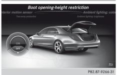
The boot lid opening limiter makes it easier to close the boot lid manually.
