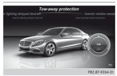
An audible and visual alarm is triggered if your vehicle's angle of inclination is altered while tow-away protection is primed. This can occur if the vehicle is jacked up on one side, for example.
