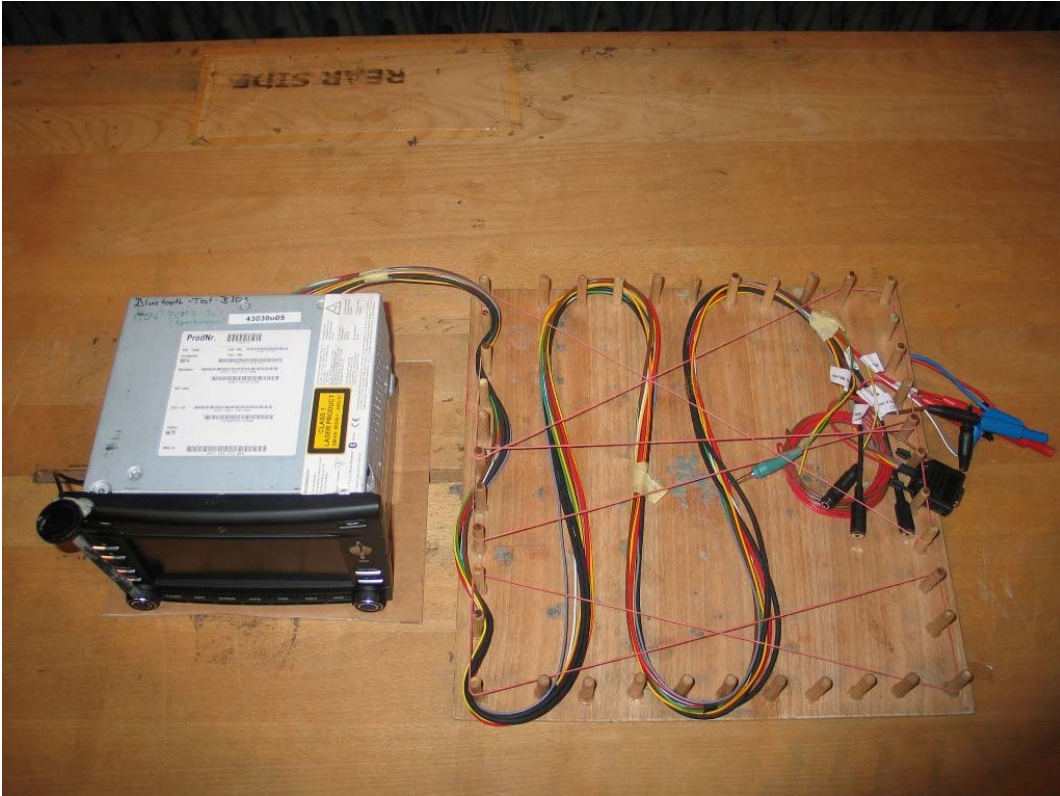
Photo 1: Test setup for radiated measurements (Enclosure, 30 MHz to 1 GHz)
