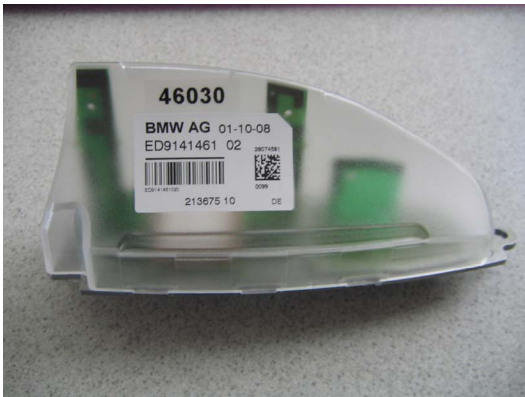
PHOTO No. 5: Ancillaries (GPS antenna)
