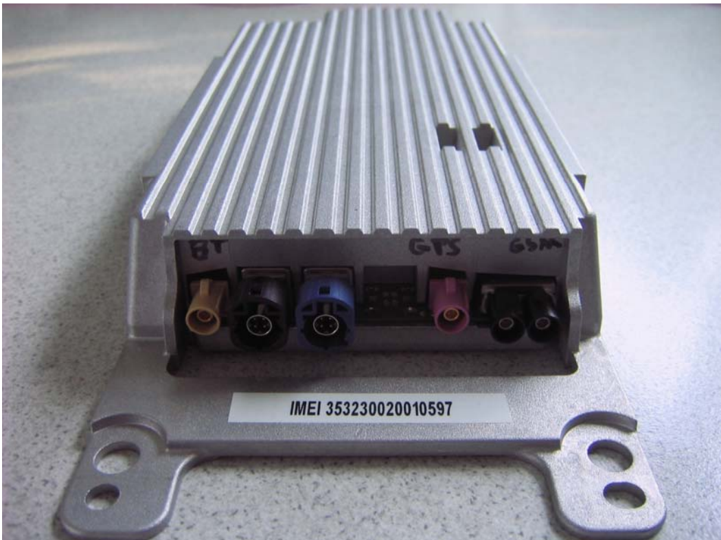
PHOTO No. 4: EUT (view on RF connectors)
