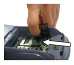
\* Keep the plastic pressed when inserting the MMC card,
