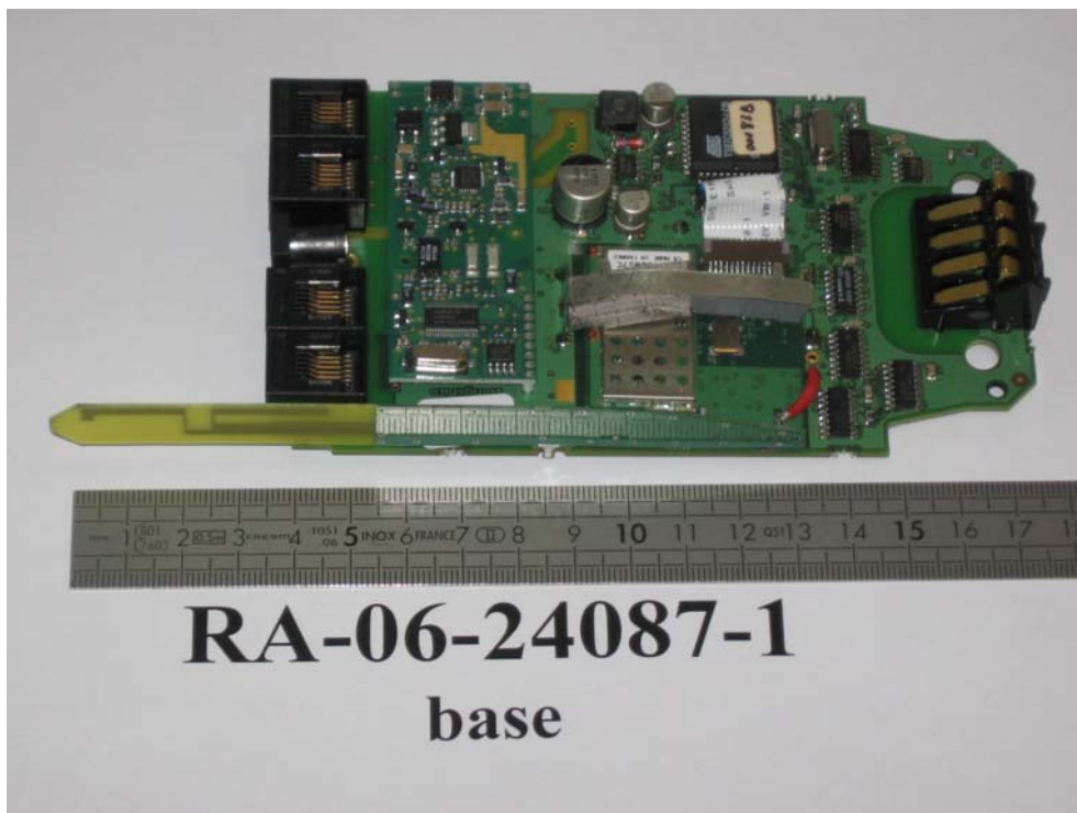
Printed circuit of the base with antenna
