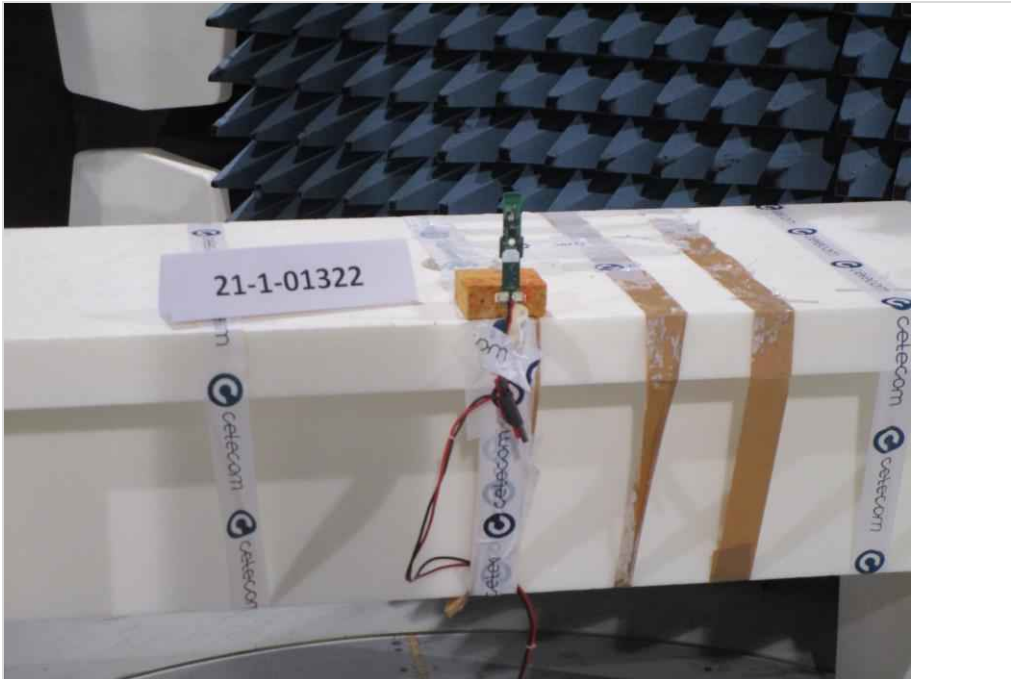
Photograph 1: EUT Test Setup in the semi anechoic chamber, Electric Field Strength
