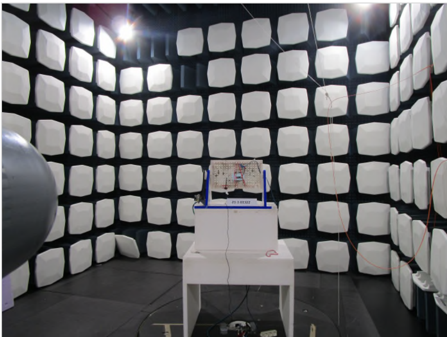
Photograph 2: Test setup in the fully anechoic chamber, overview_EUT elevation 90°, measurement >1 GHz
