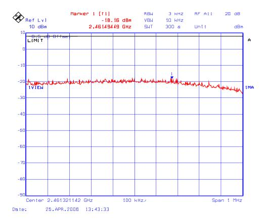
Plot # 23: Power Density in 3 kHz BW Frequency: 2412 MHz, Modulations: 802.11(b) - QPSK, Data Rate: 1 Mbps
