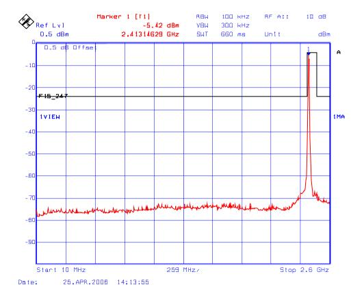
Highest Frequency: 2412 MHz, Modulations: 802.11(b) - CCK, Data Rate: 11 Mbps
