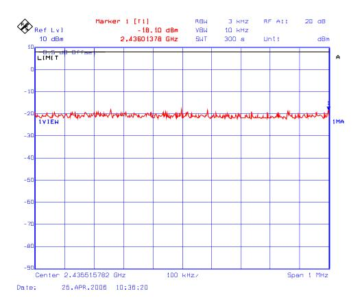
Plot # 22: Power Density in 3 kHz BW Frequency: 2462 MHz, Modulations: 802.11(b) - BPSK, Data Rate: 1 Mbps
