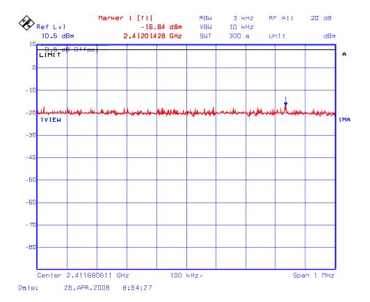
Plot # 21: Power Density in 3 kHz BW Frequency: 2437 MHz, Modulations: 802.11(b) - BPSK, Data Rate: 1 Mbps
