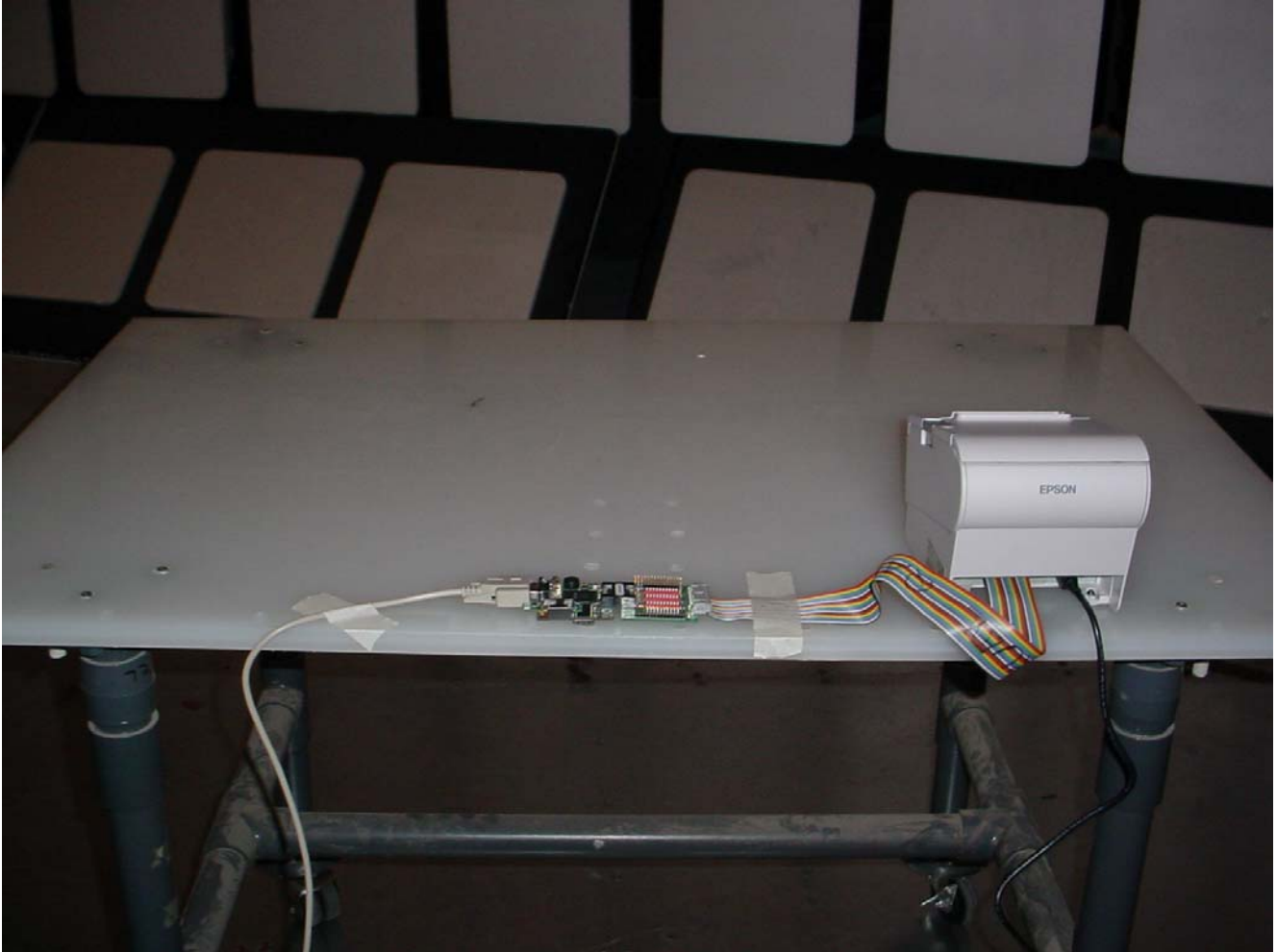
Radiated Emissions at 3 m, 30 - 1000 MHz (Orthogonal Position 1)
