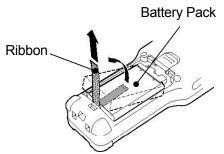
**<u>4</u>** Install a charged battery pack in the reverse order (<u>3</u> <u>2</u>).
