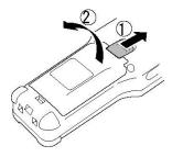
**<u>3</u>** As the following figure illustrates, pull up the battery-pack ribbon to withdraw the battery pack.
