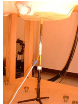
2450MHz System performance check setup
