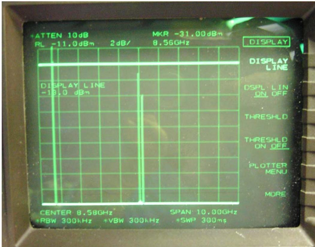
Figure 3 – Harmonics Measurement
