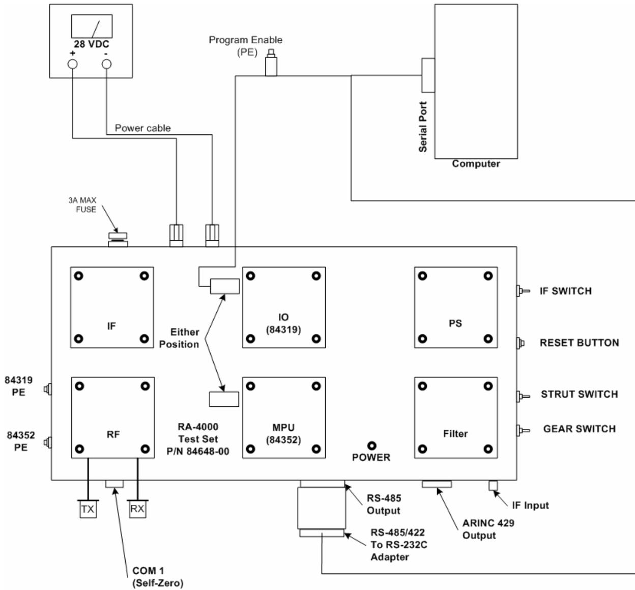
**Figure 1 – Test Fixture 84648-00**
