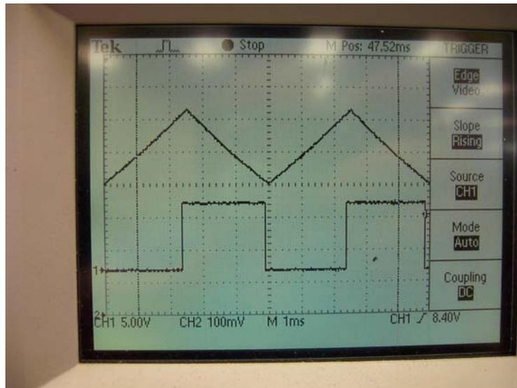
**Figure 2 – Proper Phase Lock Loop (PLL)**
