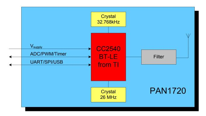
Block Diagram of PAN1721 is similar, but has I2C interface instead of USB.
