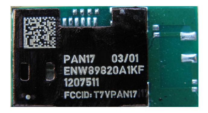
The above picture shows the full module with the case, the laser marking is made moreless on the hole case.
