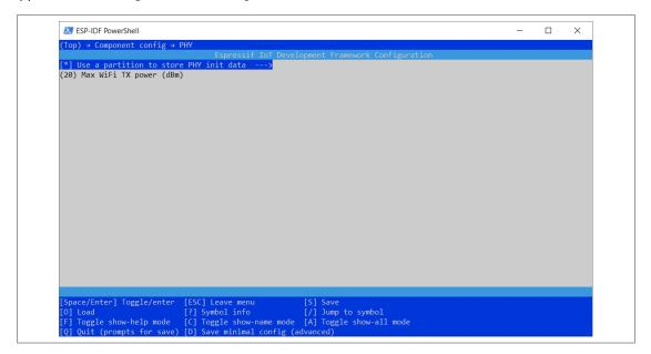
This setting will make the PAN9520 use the phy init data binary. Moreover, the default partition table will include a corresponding partition at address 0x8000, to which the binary must be flashed. Please see the ESP-IDF documentation for details: ⇒
