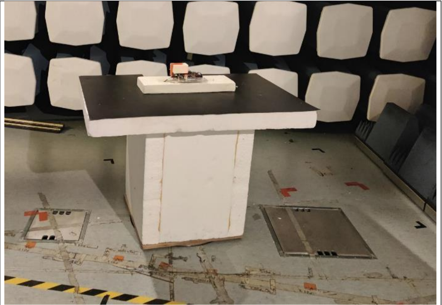
Picture 13, Radiated Spurious Emissions, EUT setup, TX and RX 30 – 1000 MHz
