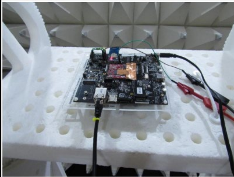
EUT Test Setup above 1 GHz-Antenna 3
